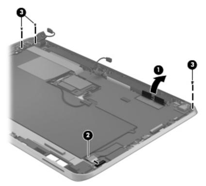
**13.** Remove the six Phillips PM1.4×2.3 screws **(1)** and the Phillips PM1.4×3.2 screw **(2)** that secure the system board to the bottom case.
